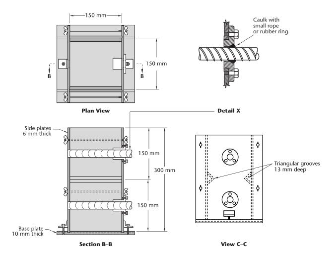
**Note:** This figure is based on a figure from ASTM Standard C 234.
