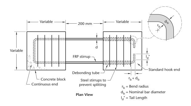
Figure E1 Configuration of Test Specimen
