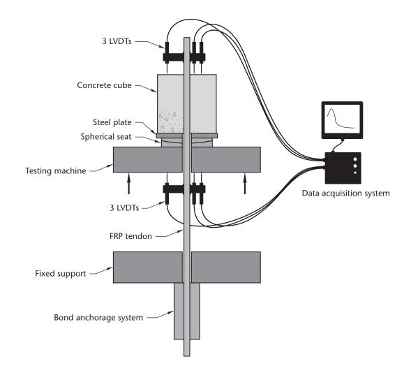
Figure H5 Bond Test Set-up
