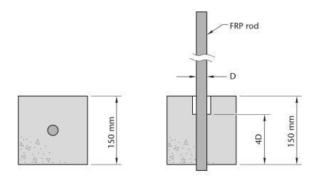
Figure H1 Vertical Bond Test Specimen (See Clause H4.1.2.)
