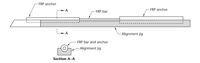
Figure B3 Jig to Align Specimen and Anchors
