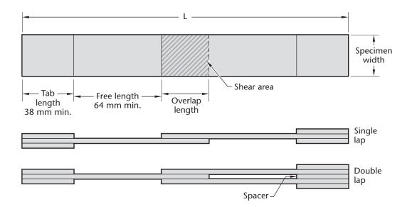
Figure Q1 Overlap Tension Specimen
