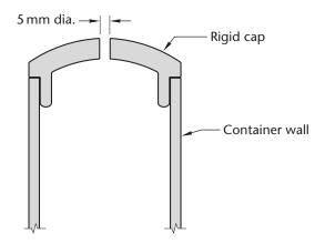
Figure A1 Specimen Container Cap
