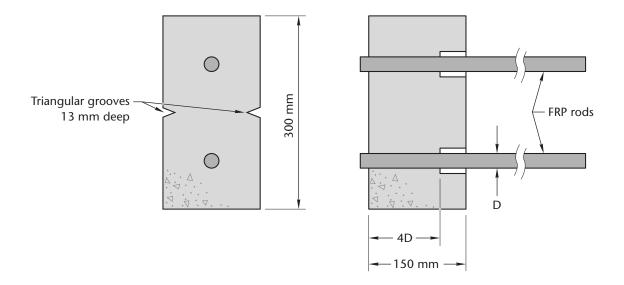
Figure H2 Horizontal Bond Test Specimen
