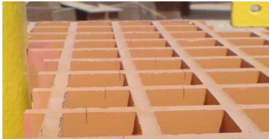
FIG. X2.4 Vertical Cracks in Molded Cells
